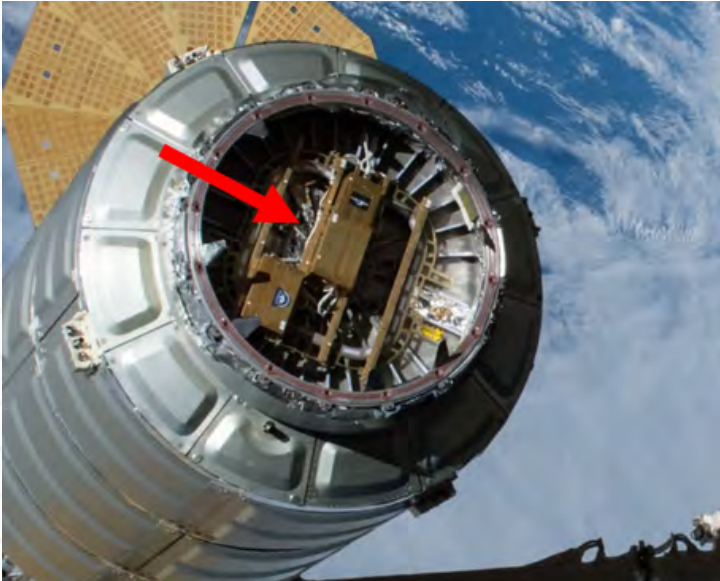
SEOPS Slingshot CubeSat deployer on the Northrop Grumman Cygnus resupply capsule. Photo credit: NASA/SEOPS.
